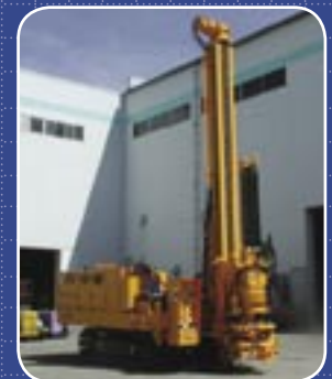
SONIC CRAWLER RIG
